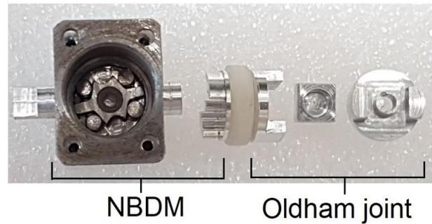
Fig. 4. Manufactured prototype of the new transmission (NBDM and miniaturized Oldham joint) for the revised version of the *S-Finger* [3].
