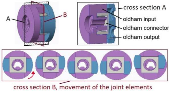
Fig. 2. Design of the miniaturized Oldham coupling joint. Top left: assembled Oldham coupling. Top right: cross section 'A' of the assembled joint. Bottom: cross section 'B' of the assembled joint showing the sliding movement of the single parts with respect to each other.
