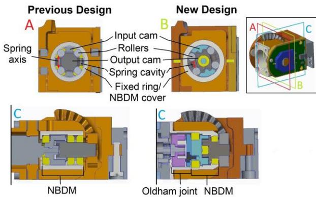
Fig. 3. Comparison between the previous and the new design of the mechanical transmission of the *S-Finger*. Top row: horizontal cross section (A, B) of the finger at the NBDM level. Bottom row: sagittal cross section (C) of the NBDM. The new design includes a miniaturized version of an Oldham coupling joint.
