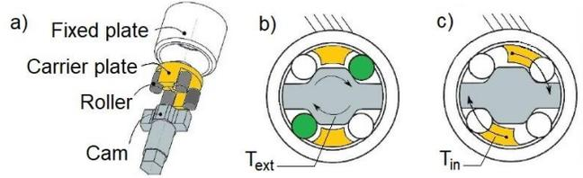
Fig. 1. Overview of the previous design of the NBDM of the *S-Finger*: A) exploded view. B) NBDM in its locked condition, cross section. The cam is forced from the output shaft (cam, gray) by an external torque  $T_{ext}$  resulting in wedged rollers (green) preventing the rotation of the cam. C) NBDM in its unlocked condition, cross section. When the motor is driven, the torque  $T_{in}$  is transferred to the carrier plate (yellow) unlocking the rollers. (Adapted from [3]).
